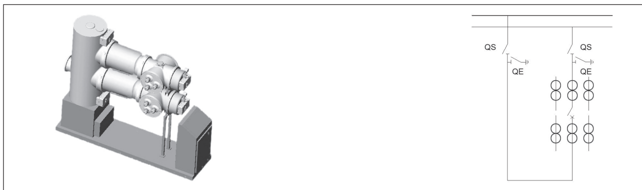
双母线套管进出线间隔1/Bushing incomer/feeder bay of double busbar 1
