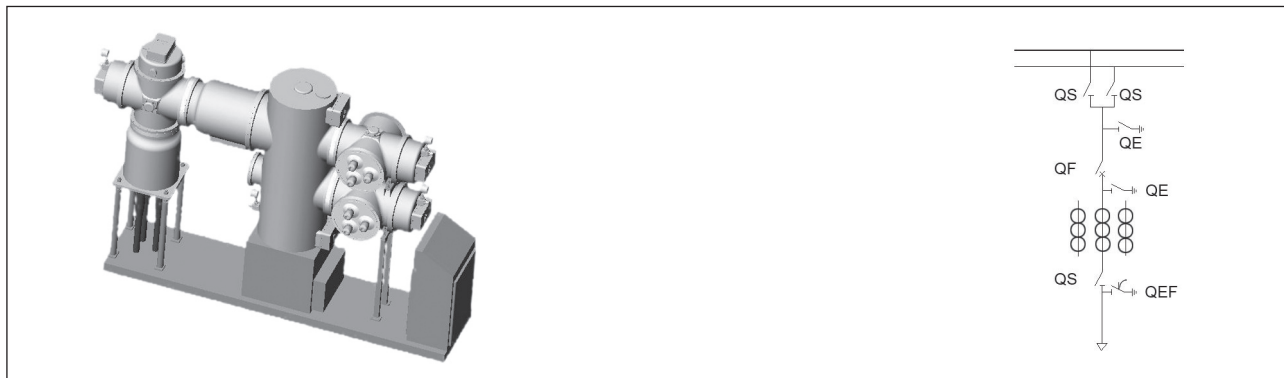
母联间隔/Busbar coupler bay
